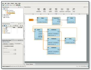
The Alarm Notification Pipeline in Ignition software allows for easy drag-and-drop alarm configuration.
